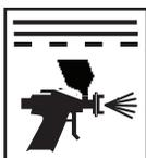
Using 25 - 30 psi, apply 2 - 3 wet coats of the mixture. Allow a 10 - 15 minute flash period between coats at 21° C / 70° F. \*The flash time between coats will vary depending on the amount of material applied, temperature, and air flow.
